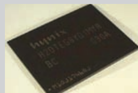
E2NAND Product Specifications Package LGA 52 / 2 Channels Capacity 16GB (1+4-stack) / 32GB (1+8-stack) 64GB (8-stack)
